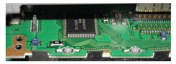
**Above:** One bank of LEDs shown with the series resistor ("151"). The anode of the diode (long lead) is on the same side as the resistor (left) for both LEDs. Make sure all 6 diodes are orientated this way! Also the LED leads must be bent back as shown. Make sure the LED sits all the way down into the hole.
