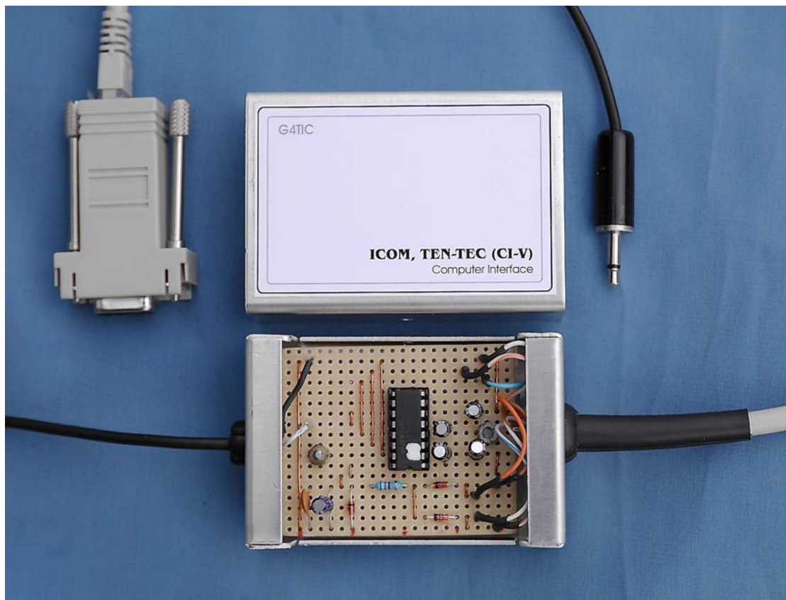
The finished ICOM interface
