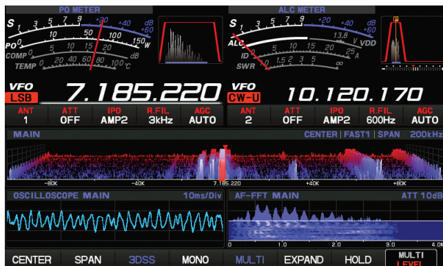
Figure 4 — In this view, the 40-meter RF spectrum is shown and below that, the received audio is shown with both oscilloscope and spectrum analyzer views.
