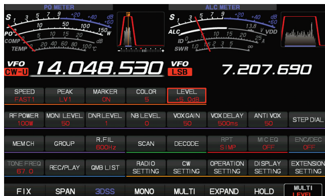
Figure 5 — Pressing the FUNC button (below the screen) opens up the top menu display. The MULTI button is used to select the desired function, and then pressing the MULTI button brings up the adjustable parameter, or an additional layer of menu items.
