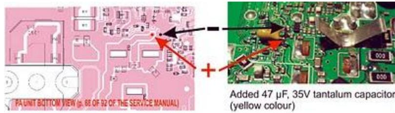
This step requires adding an extra tantalum bypass capacitor across C305 (470µF, 16V) (PA UNIT). Locate the capacitor's leads (see photo and schematic diagram) and solder a **47 µF / 35V** tantalum capacitor across the electrolytic. **Observe the polarity!!**
