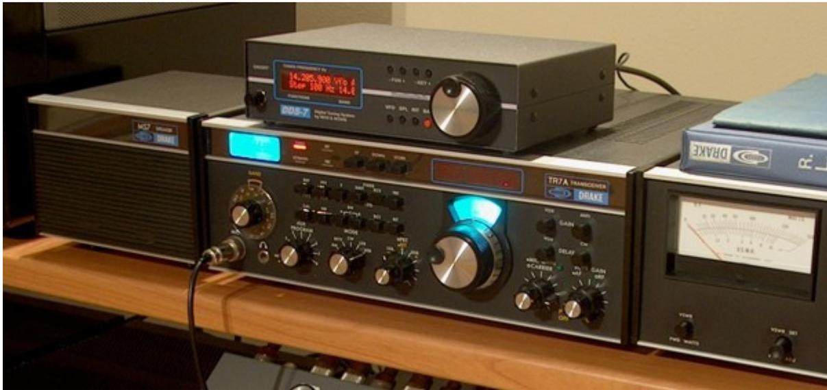
DDS-7 substitute all the original tuning system of TR7, generating a frequency range required by first MIXER in UP-CONVERTER module. The signal generated from 48.050 to 78.050 KHz. is applied to this module and the original signal generated by VCO/PTO units is disable. At this point the tuning is performed by DDS-7, the VCO/PTO are active but disconnected, the original RIT function is disable and performed by DDS-7 only.
