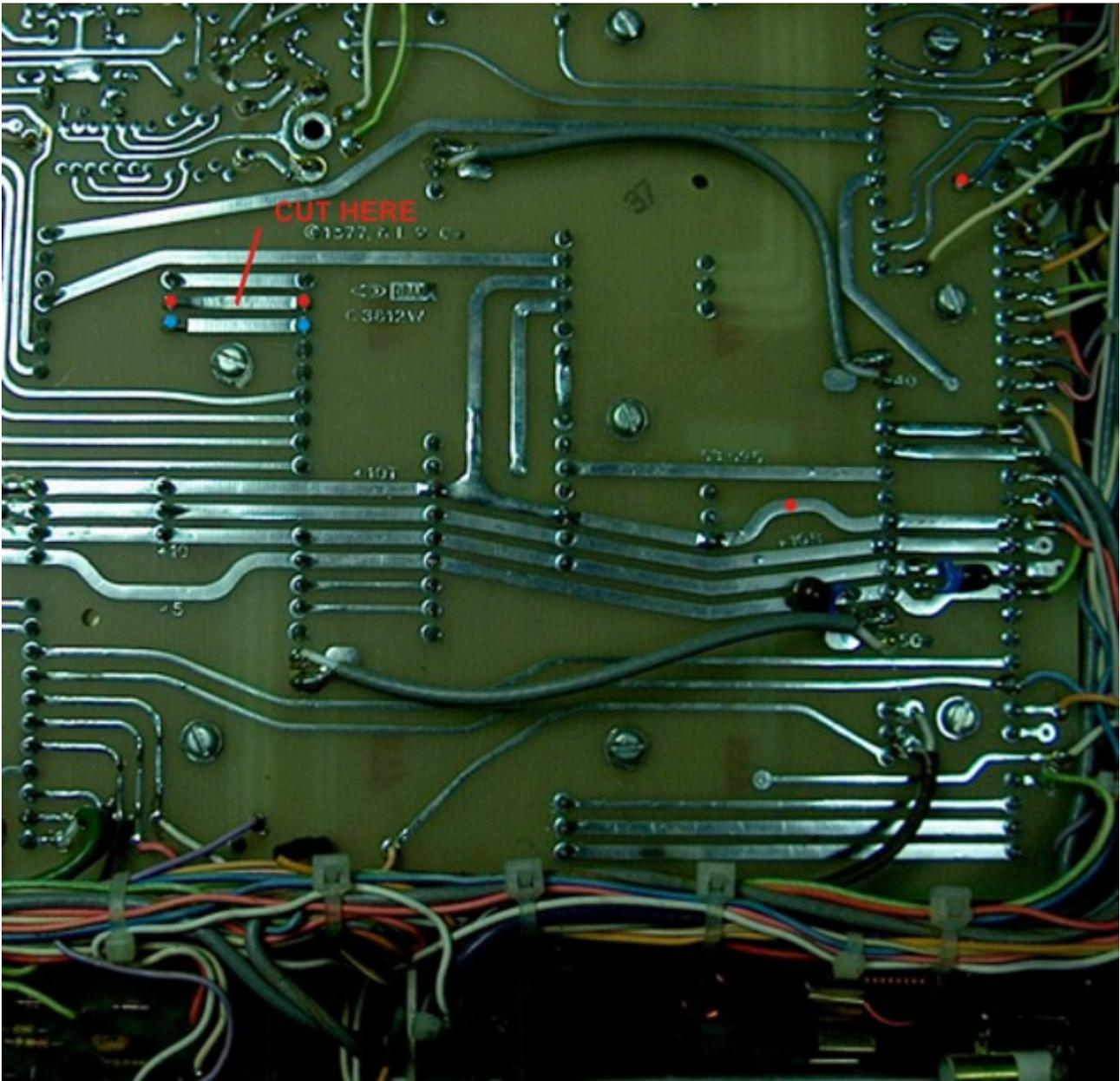
This is the bottom of the main PCB BUS of TR7, access it removing the bottom enclosure's panel after the main slide top cover.
