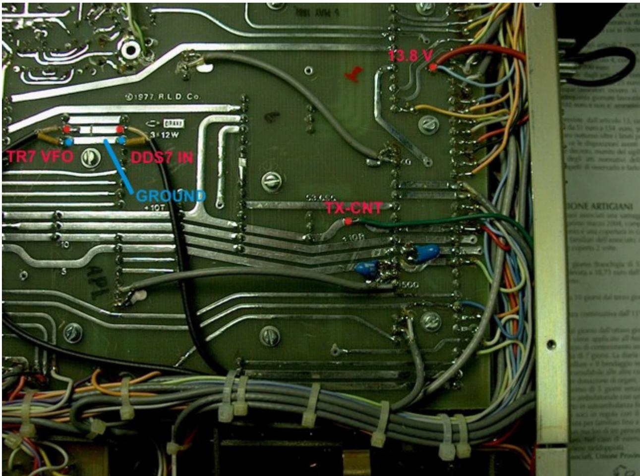
Solder the two coax cable coming from connections box to the indicated positions by the RED and BLUE dot:
