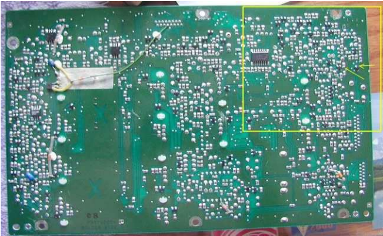
The resistor chip to be removed.
