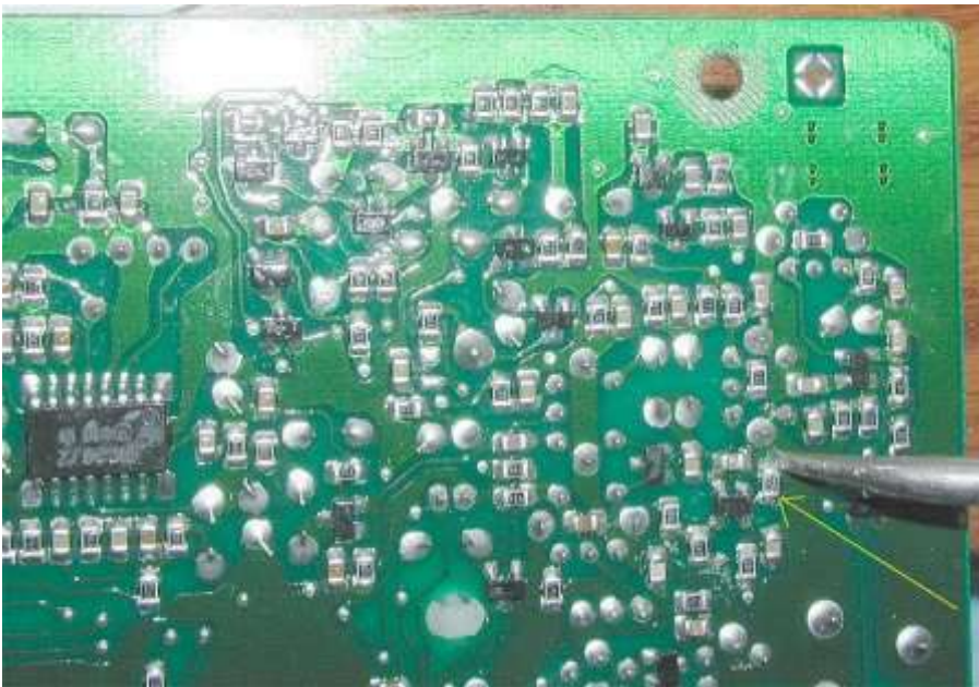
The modification with a 220 ohm resistor to switched ground.
